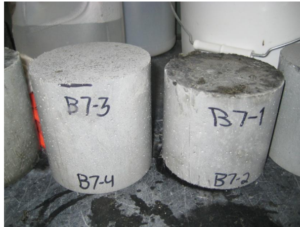
Figure 3.2. Diamond Cut and Rough Top Surface Finishes
