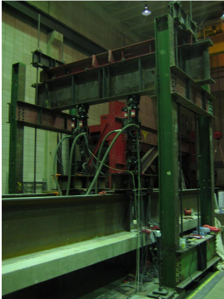
Figure 3.21. Load Frame for Service Level Testing
